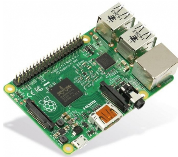
Abbildung 4.1: Raspberry Pi Version 2 Model B
